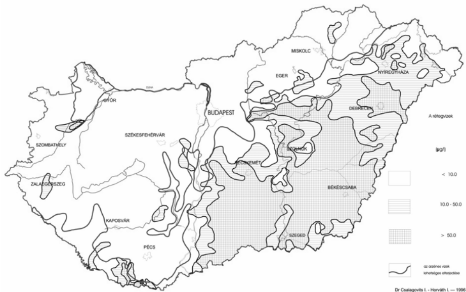
Fig. 2. Pleistocene layer thickness and arsenic water (after Csalagovits, 1996)
